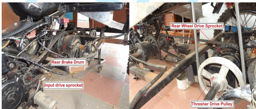
Fig. 6 Power Unit Transmission System
