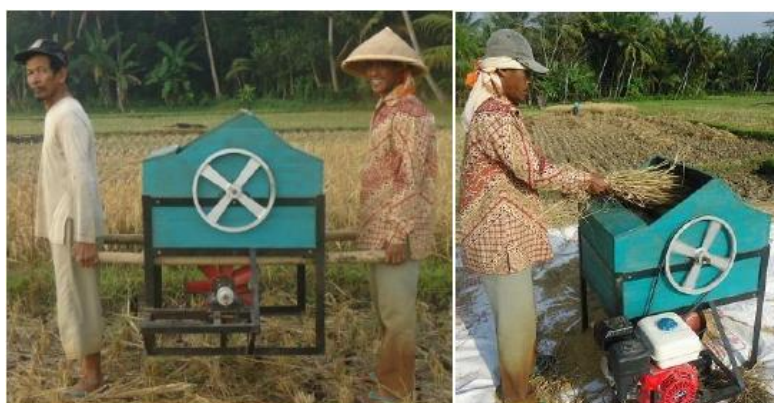
Fig. 3 Steel and wood rice thresher (Kristanto. A. et al, 2015)
